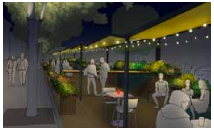
Step 06 | Different levels of lighting, including uplighting of trees, catenary lighting and individual table lights bring further quality.
