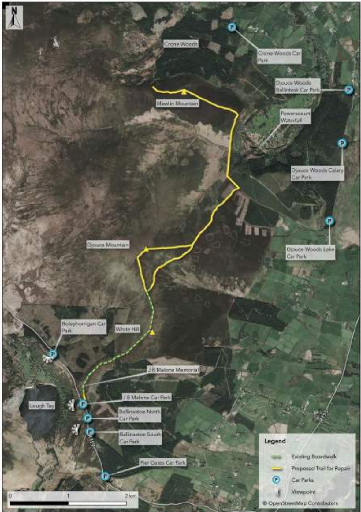
Fig. 16 Path erosion works required on Djouce and Maulin.
