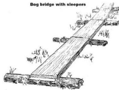
Figure 18 Simple bog bridge structure with sleepers
